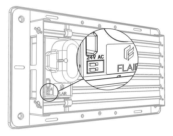
24VAC Optional Power Port Use with: 20AWG Plenum Rated Solid 2 Conductor Wire @24VAC: less than 1mA continuous, max 50mA Intermittent
